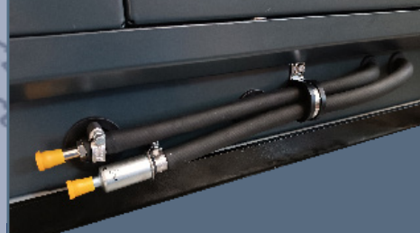
INPUT/OUTPUT FUEL PIPE
