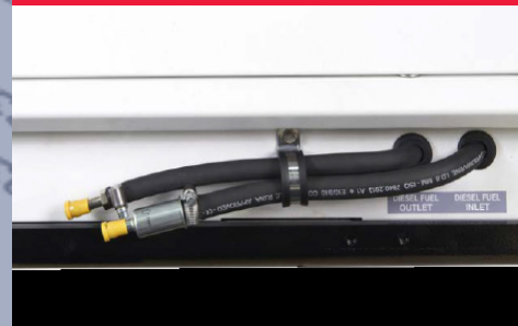
INPUT/OUTPUT FUEL PIPE
