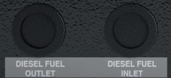
INPUT/OUTPUT FUEL PIPE
